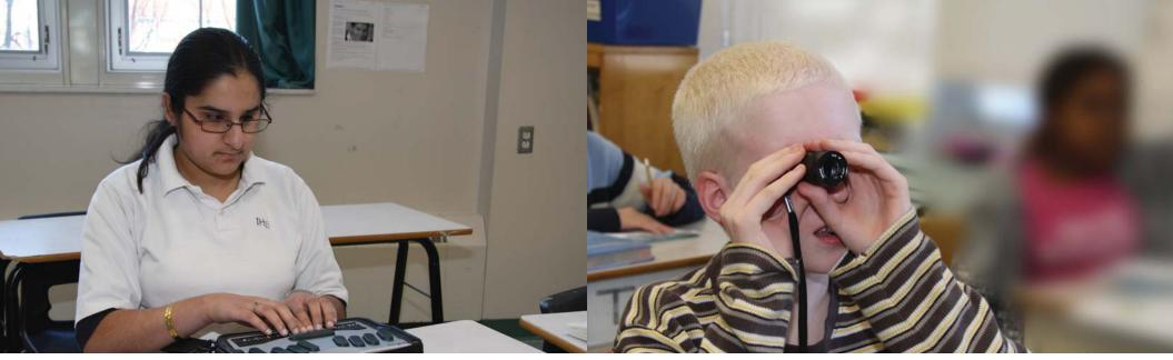
A portable electronic braille notetaker allows a student to braille and save documents that can later be downloaded onto a computer.
